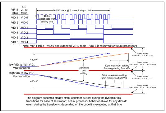
The processor load may not be sufficient to absorb all of the energy from the output capacitors on the baseboard, when VIDs change to a lower output voltage. The VRM/ EVRD design should ensure that any energy transfer from the capacitors does not impair the operation of the VRM/EVRD, the AC-DC supply, or any other parts of the system.
